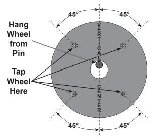
b. Tap the flat side of the wheel with a light non-metallic object, such as a screwdriver handle, at a point 45° from the vertical center line on each side of the wheel and 1 – 2 inches from the edge of the wheel (see Il-lustration).
